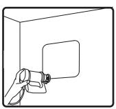
**2.** Use provided cutout template to mark hole. Use RotoZip or other tool to cut hole in wall. Hole size: 4 in. (102 mm) tall x 4 in. (102 mm) wide.
